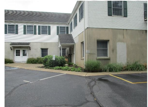
Downspout planter boxes can be constructed at the northeastern downspout. Pervious pavement can be installed along the eastern edge of the parking lot to capture, treat, and infiltrate stormwater runoff from the roof and parking lot. A preliminary soil assessment suggests that more soil testing would be required before determining the soil's suitability for green infrastructure.
