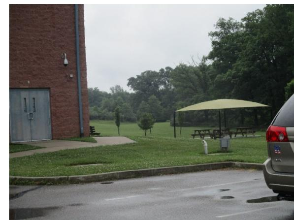
A rain garden can be installed south of the gym building to capture, treat, and infiltrate stormwater runoff from the roof. The nearby downspouts can be disconnected into the rain garden. Parking spaces west of the gym can be converted to porous pavement to capture and infiltrate stormwater runoff from the parking lot. A preliminary soil assessment suggests that more soil testing would be required before determining the soil's suitability for green infrastructure.
