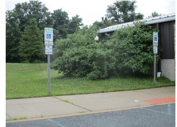
A rain garden can be installed west of the building to capture, treat, and infiltrate stormwater runoff from the roof. The nearby downspout could be disconnected to capture rooftop runoff into the rain garden. A preliminary soil assessment suggests that more soil testing would be required before determining the soil's suitability for green infrastructure.
