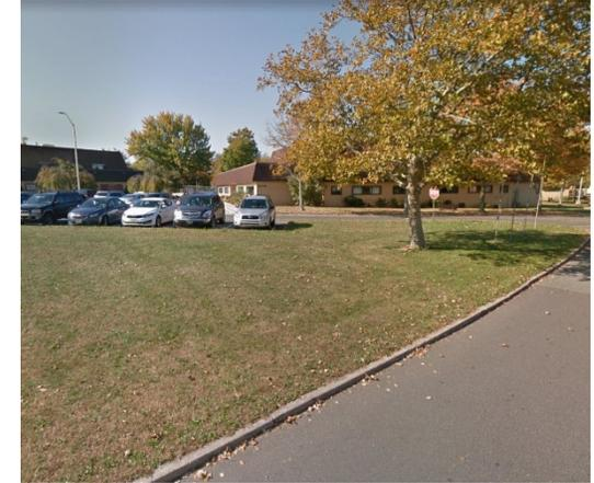
A rain garden can be installed in the north of the eastern parking lot to capture, treat, and infiltrate stormwater runoff from the parking lot before reaching the nearby storm drain. A preliminary soil assessment suggests that the soils have suitable drainage characteristics for green infrastructure.
